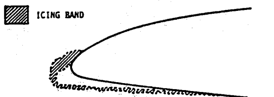
b) Composite of ice shape tracings showing icing band
